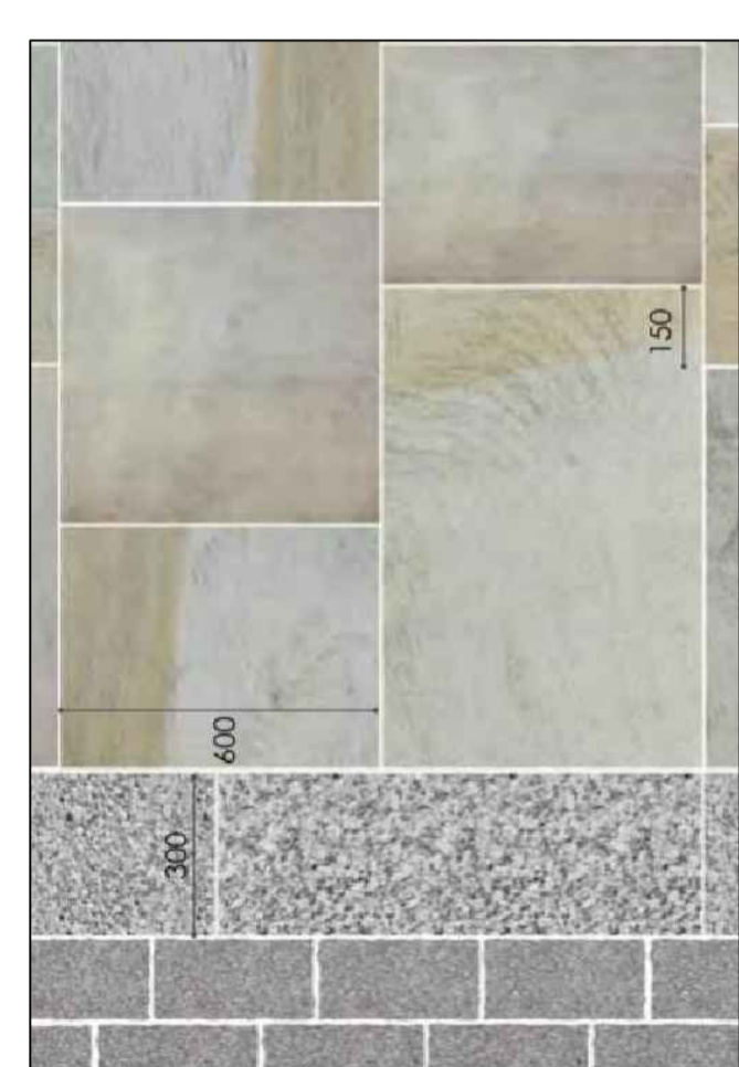
New paving - Yorkstone with granite kerbs
